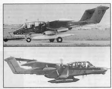
Agile, capable, field-maintainable, the OV-10 proved itself an excellent closesupport combat craft from Vietnam to the Gulf War. Top photo of "155477" shows original OV-10A configuration at roll-out during 1969 Paris air show. Bottom photo is of same plane modified to OV-10D specs, over Ohio in 1980. Photos: Norman Taylor Collection
